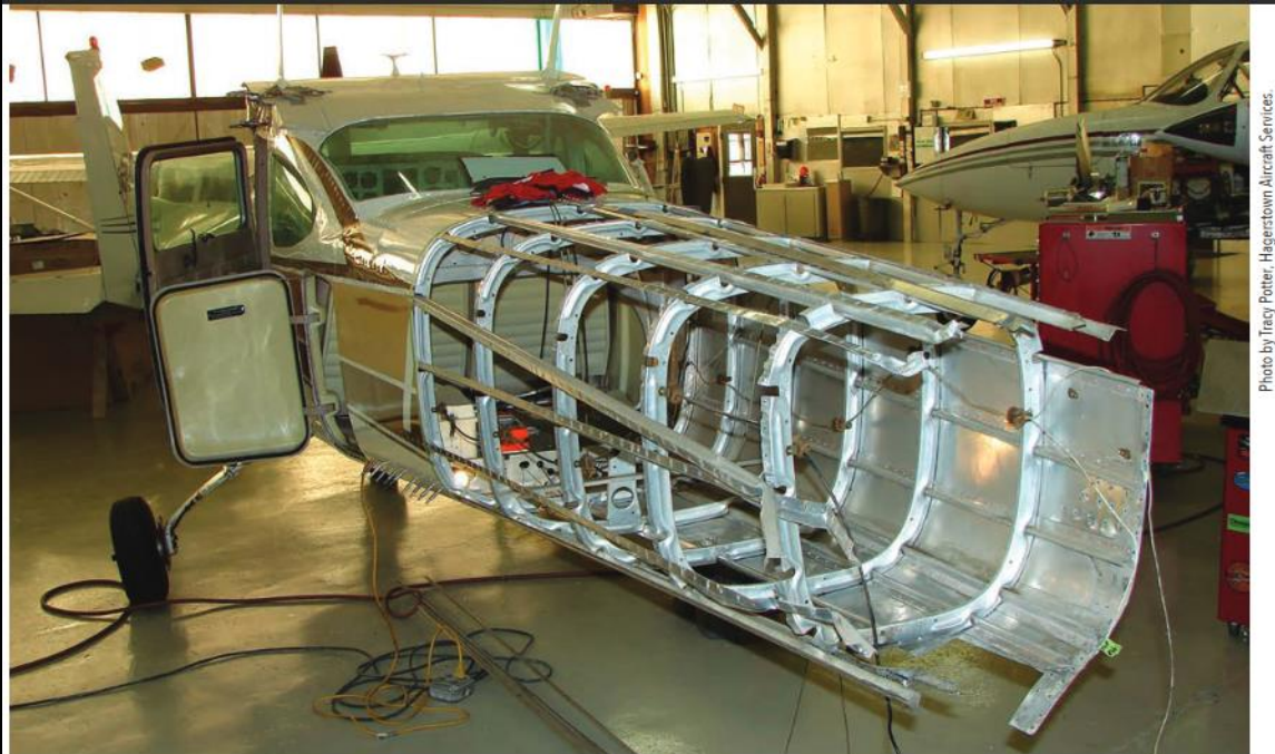
The internal construction of a semi-monocoque airplane showing damage from a wildlife strike.
