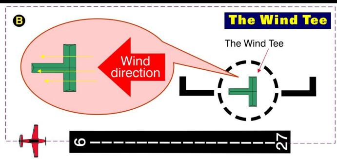
The wind tee is free to rotate into the wind. Think of its shape as an airplane that points in the direction you should land (into the wind). The wind tee may be manually rotated by airport personnel to identify the proper landing direction. It may also be tethered, unattended and completely inaccurate! Use caution when using it to assess landing direction.
