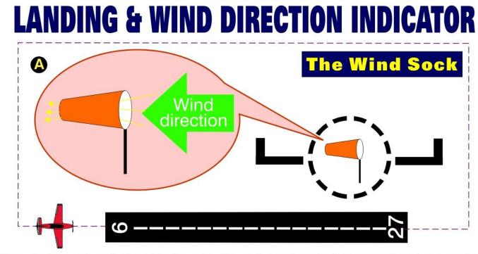
The wind cone (or wind sock) aligns itself parallel to the wind. The small end or opening points downwind and the big end (the opening) is upwind. To decide on wind direction, simply look at which way the small end points. This is the direction the wind is blowing. You'll land into the wind. © Rod Machado's
