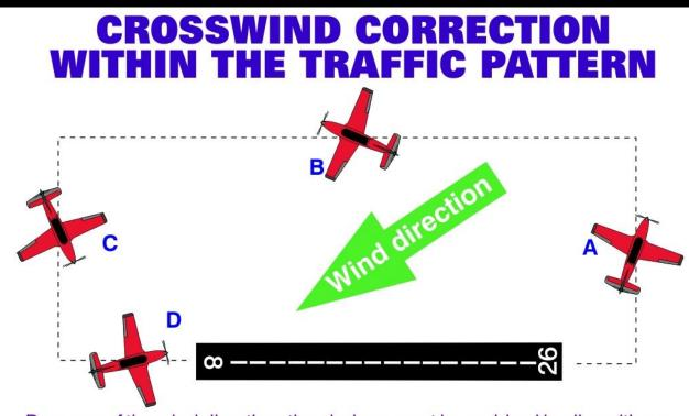
Because of the wind direction, the airplane must be crabbed in all positions, (A, B, C, & D), to maintain a rectangular traffic pattern.
