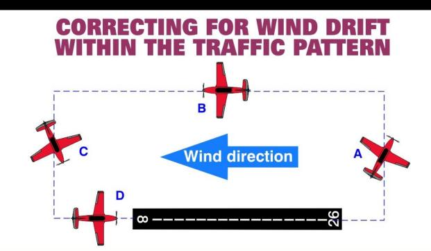
In positions A & C the airplane crabs (points) into the wind to maintain a rectangular ground track in the traffic pattern. The stronger the wind, the greater the crab angle needed to fly a rectangular ground track.
