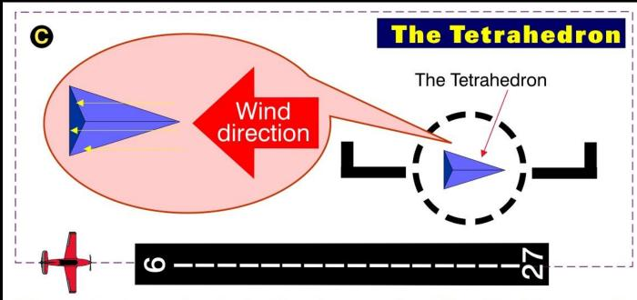
The tetrahedron points in the direction you should land (or it is manually pointed in the direction you should land). It is mounted on a swivel and can pivot, and like the wind tee, its reliability is questionable during light winds.
