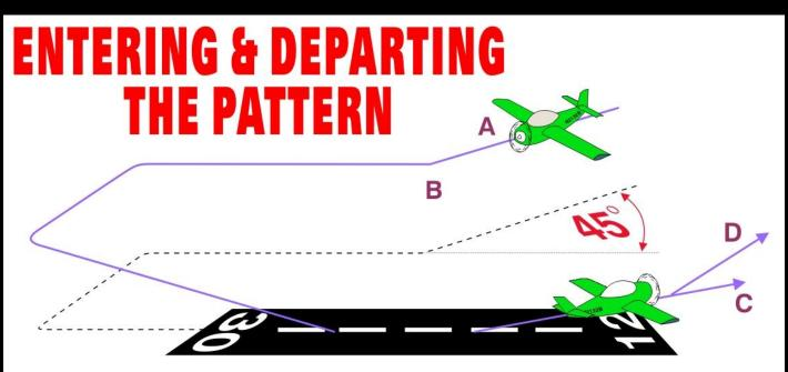
Enter the traffic pattern at a 45 degree angle (A) to the downwind leg about midfield (B). When departing an airport, make either a straight out (C) or a 45 degree turn in the direction of the pattern (D) when reaching pattern altitude.
