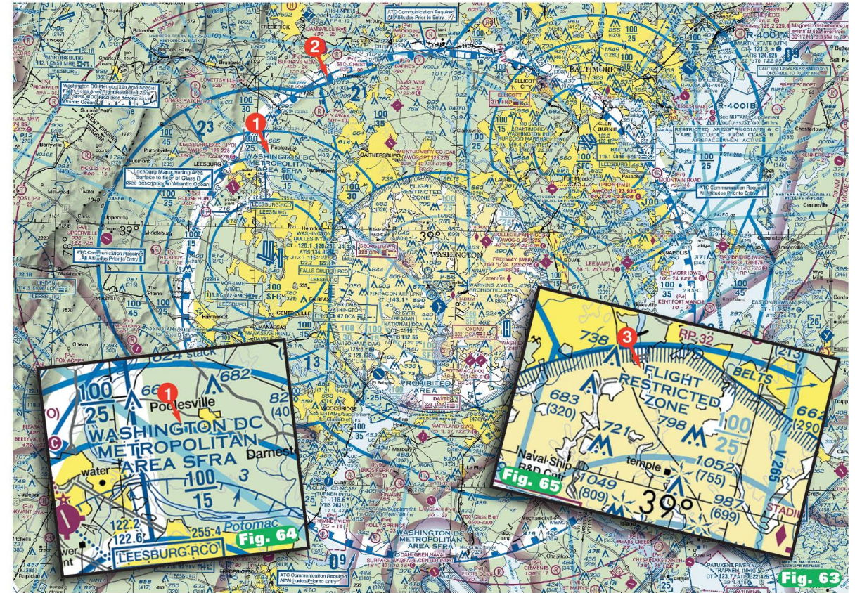
Flight Restricted Zone (FRZ), Special Flight Rules Area (SFRA) in Washington, D.C. Airspace
