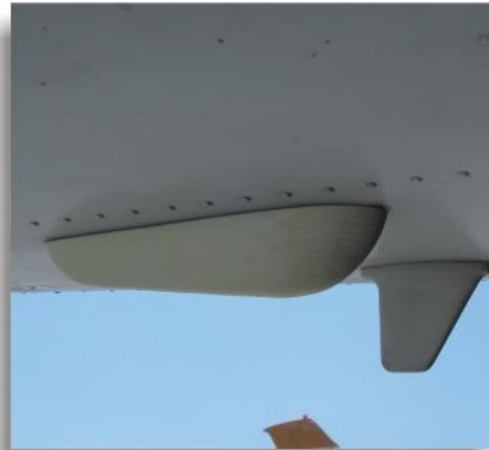
Marker Beacon Antenna
